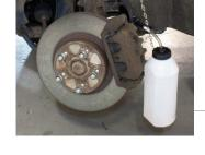
WASTE FLUID BOTTLE CONNECTS TO VEHICLE'S BLEEDER SCREWS AND CHAIN WITH HOOK HOLDS BOTTLE IN PLACE.
