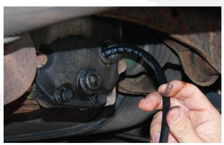
FLEXIBLE ADAPTERS FIT IN ALL DIFFERENTIAL OPENINGS.
